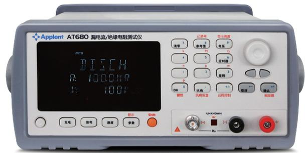
■ Power Supply 198VAC~252VAC 47.5~52.5Hz Power: maximum 50VA
