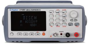
Power Supply 198VAC-252VAC 47.5-52.5Hz Power: maximum 50VA
